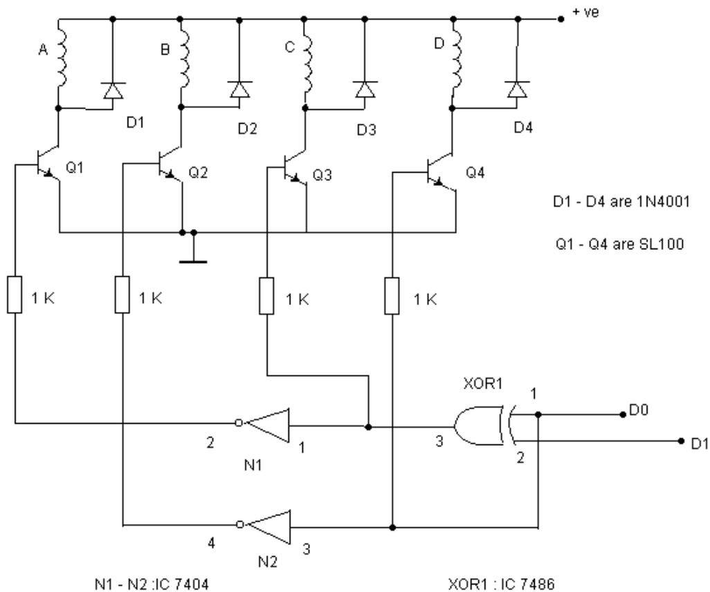
PINS 14 & 7 of both the ICs are to be connected to +5V and Ground respectively.
